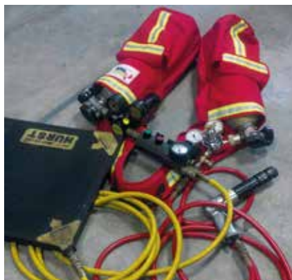
▲ The KrusePak can be utilized in multiple operations on the fire ground including Rescue/Extrication operations when utilizing air bags or an air chisel.
